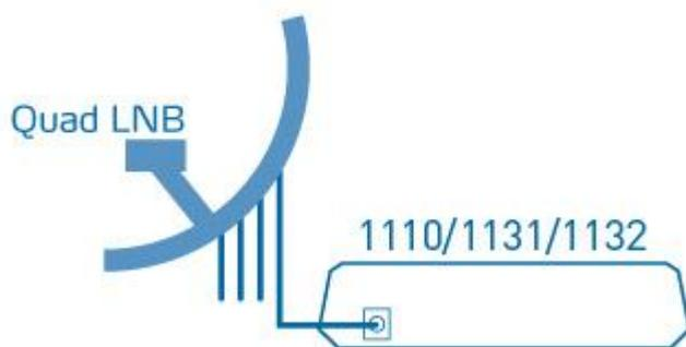
Connect any one of the four cables from the satellite dish directly to the LNB input on the back of the device.
