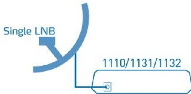
Connect the cable from the satellite dish directly to the LNB input on the back of the device.
