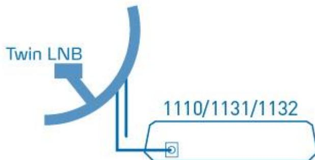
Connect either cable from the satellite dish directly to the LNB input on the back of the device.
