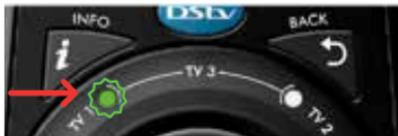
To set the remote to TV1 mode: press and hold the **i** button for 3 seconds or until you see the **green** light blink on TV1 (below the **i** button).
