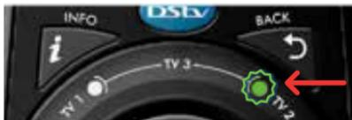
To set the remote to TV2 mode: press and hold the **BACK** button for 3 seconds or until you see the **green** light blink on TV2 (below the **BACK** button).
