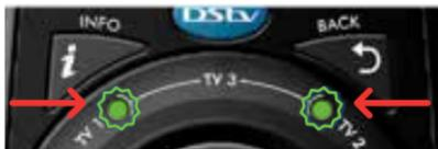
To set the remote to TV3 mode: press and hold both the **i** and **BACK** buttons for 3 seconds or until you see the **green** light blink on TV1 and TV2 (below the **i** and **BACK** buttons).
